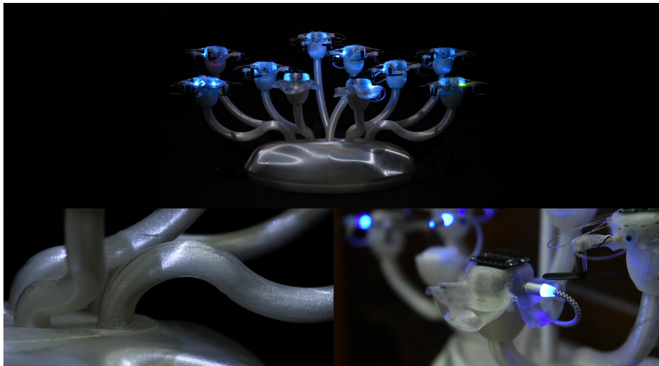
Figure 2: How to Train your Drone. Top: The charging station with the different drones and hand-sensors docked on top. Bottom left: The 3D printed material of the charging station. Bottom right: The hand-sensors that can be attached to the hands.
