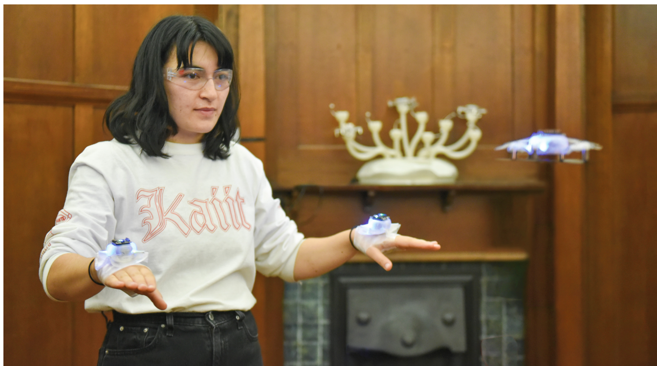
Figure 1: How to Train your Drone: Nora, one of our co-creators, wears hand sensors while flying the drone. The charging dock rests on the mantel in the background.
